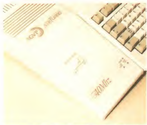
GVP's A530 can make your A500 faster than an A1200, but it won't give you AGA graphic support.
